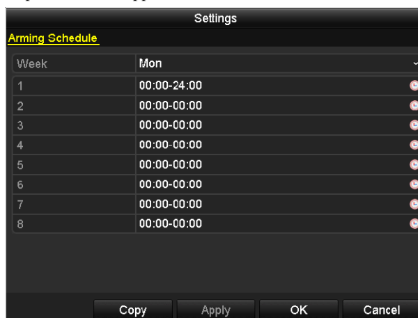
Figure 8. 24 Set Arming Schedule of Alarm Output
